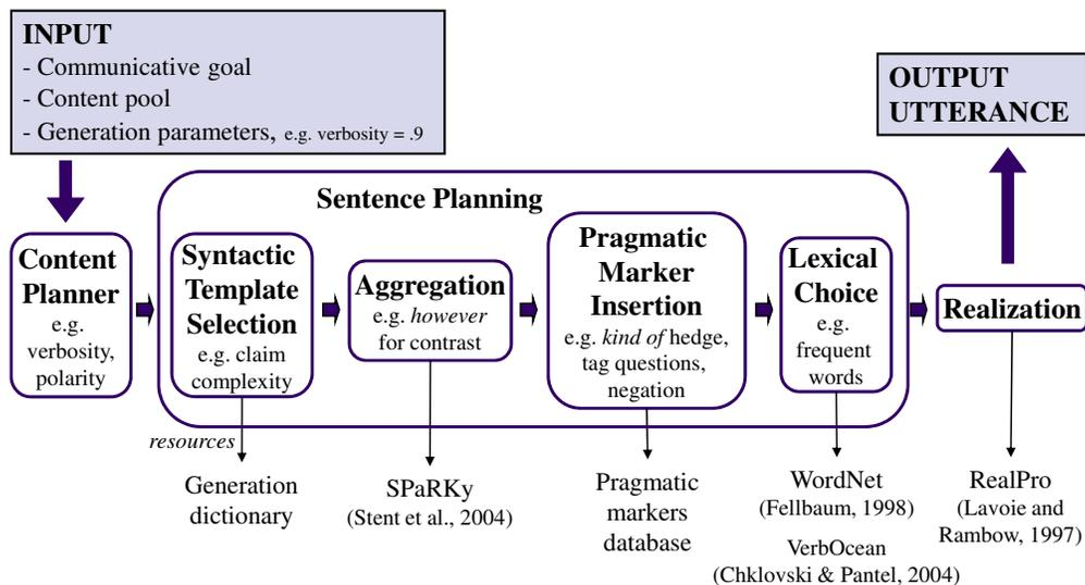
Fig. 2: The architecture of the PERSONAGE base generator.
